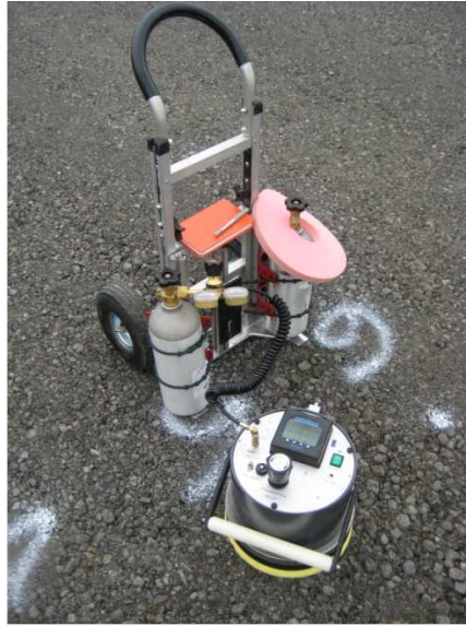
Figure 4. Gas permeability test used in the field
