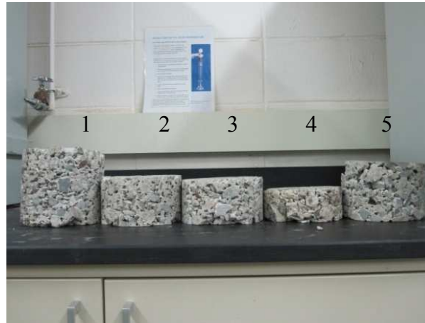
Figure 100. Compaction of specimens of CTB I-96 Michigan
