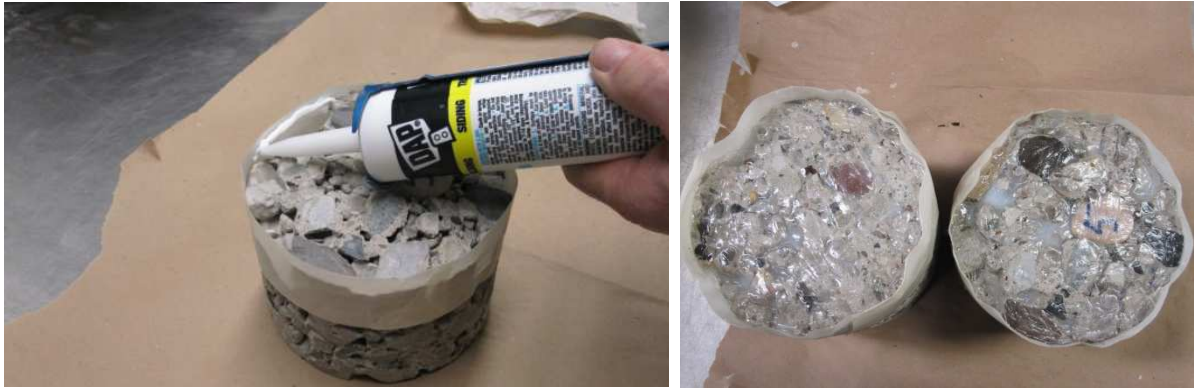
Figure 101. Sealing the bottom of CTB of I-96 Michigan
