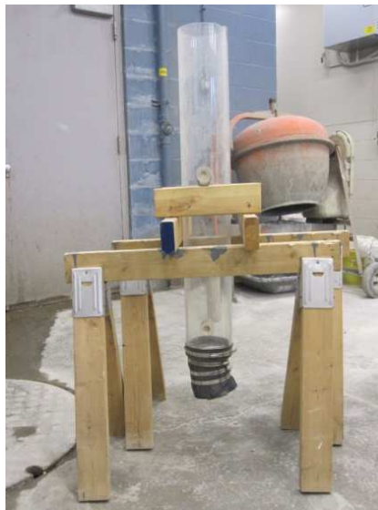
Figure 11. Falling Head Permeability Testing of cement treated base
