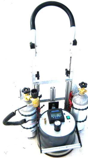
Figure 134. Gas Permeameter Test (GPT) Device
