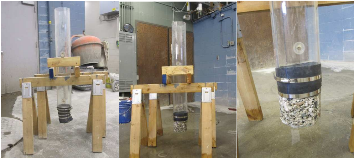
Figure 102. Falling head permeability test of vertical flow (left) and horizontal flow (middle and right) of CTB, I-96 Michigan
