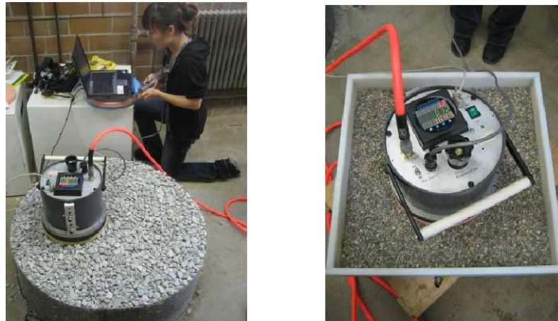
Figure 103. Laboratory GPT tests in 0.95 m diameter by 0.31 m height ring (left) and 0.57 m square by 0.15 m height box (right)
